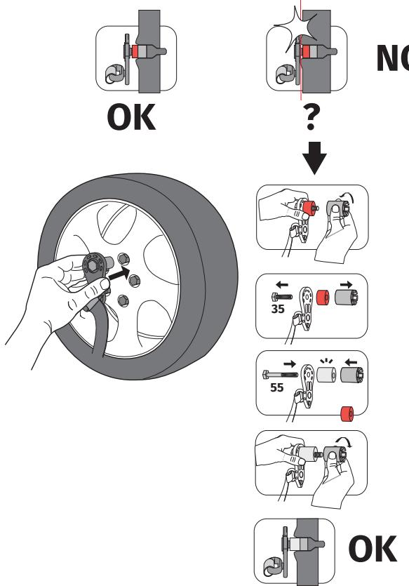
**EN In case the problem is not solved, configure the fixing system as shown here below.**
