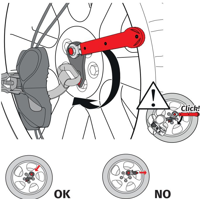
**EN Insert the tool on the screw hex head and torque until the tool clicks. Check that after screwing the red arrow is directed towards the center of the wheel. The K-Lock tool is preset to provide the minimum torque level for wheel bolts in different sizes and geometries.**
